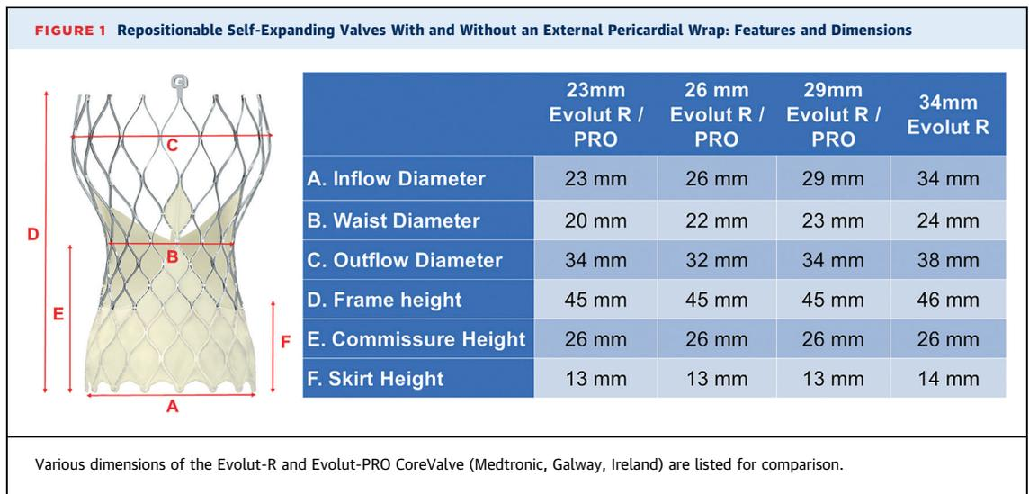
2. The concave central portion allows the frame to avoid contact with the coronary ostia.
